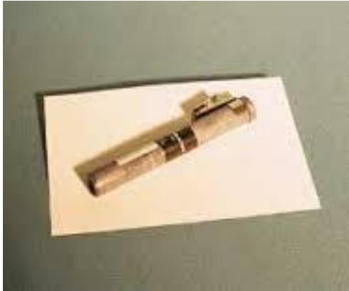
Detection – Gamma and x-ray radiation
