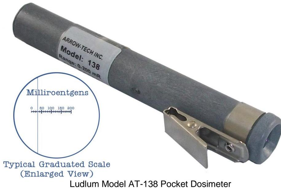
Detection: Gamma and x-ray radiation
