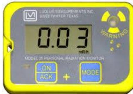
Detection: Gamma and X-Ray radiation
