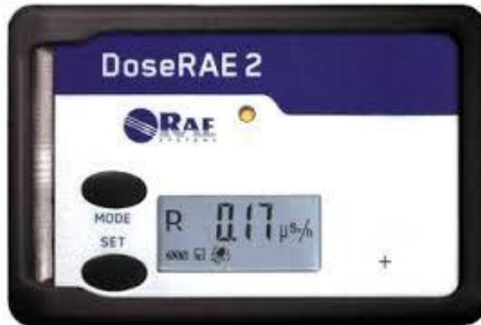
Detection: Gamma and X-Ray radiation
